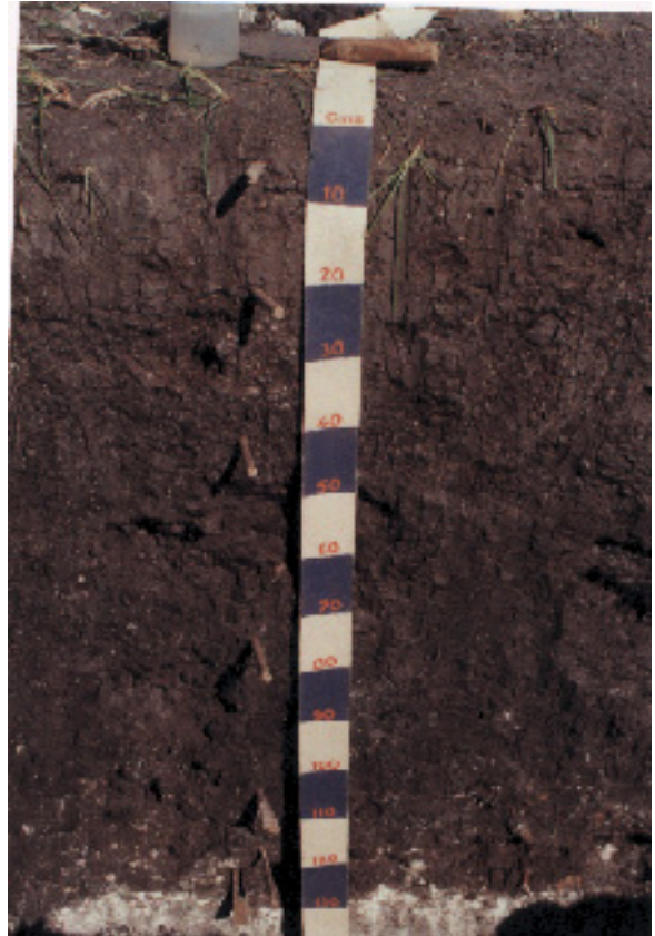
Typical black soil profile of Kovilpatti series showing accumulation of Gypsum in the lowermost horizon.
